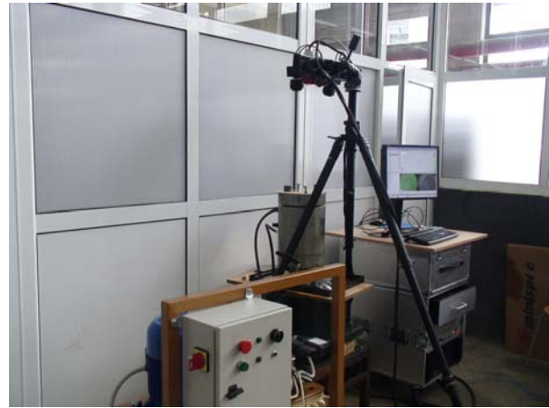
Figure 5. Experimental equipment for FLC determination.
